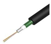
Fiber indoor/outdoor drop cable, LSZH, Gel-filled Central Tube, CST, 24 fiber, Singlemode G.652.D and G.657.A1, Meters jacket marking, Black jacket color
