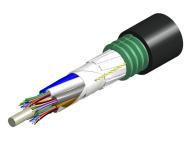
Fiber indoor/outdoor cable, loose tube gel-filled CST, 48 fiber, Multimode OM3, Meters jacket marking, Black jacket color
