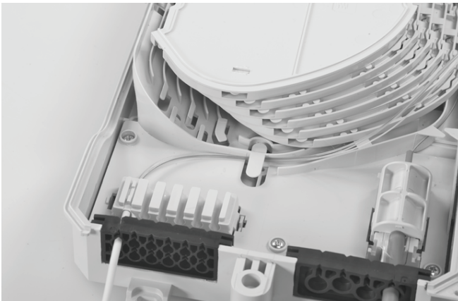
4.6 Cut the aramid yarn and close the holder with the cover.
