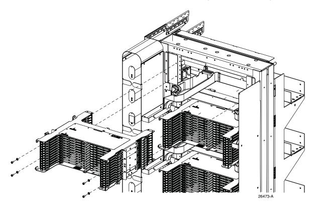
Figure 2. Installing Chassis in Frame
