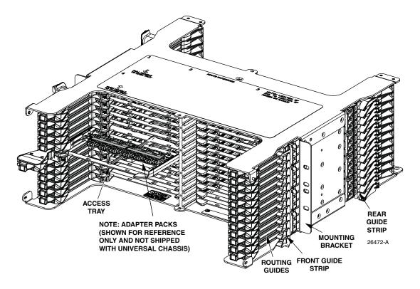
Figure 1. Main Components of NG4access Universal E-Series Chassis
