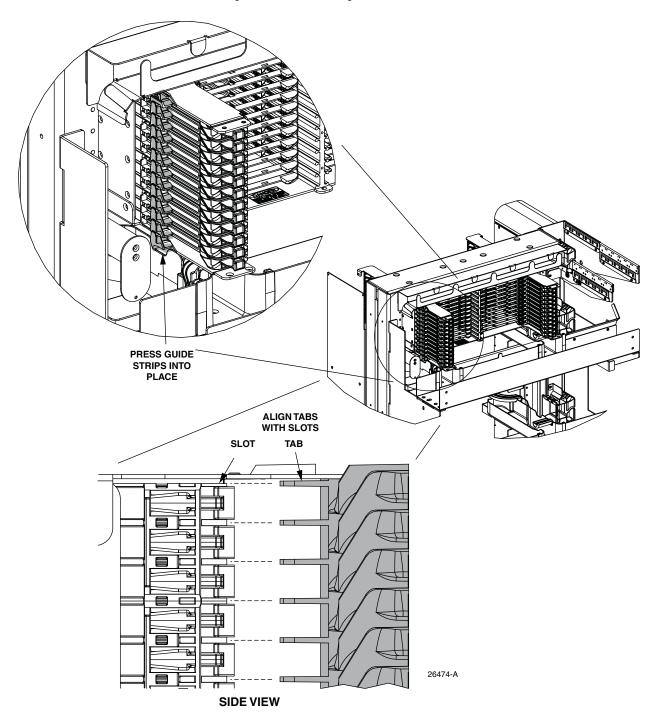
Figure 3. Installing Guide Strip On Universal E-Series Chassis
