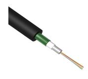
Fiber OSP cable, 12-fiber, OS2, HDPE, loose tube, 12 fiber, gel-filled, Singlemode G.652.D and G.657.A1, 1000 m, Meters jacket marking, Black jacket color
