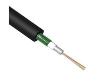
Fiber OSP cable, 4-fiber, HDPE, loose tube, gel-filled, Singlemode G.652. D and G.657.A1, Meters jacket marking, Black jacket color, 1000 m, black. Provides Rodent Resistance
