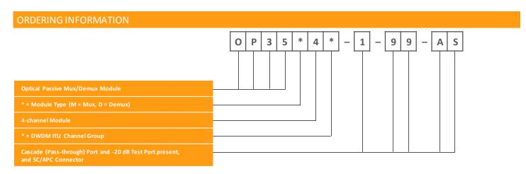
Mux and demux modules are available for Channel Groups J, K, L, M, N, P, R, S, T, and U. Please refer to the ARRIS DWDM ITU Grid Channel Plan data sheet for a complete description of the channels included in these groups.
