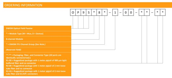
8-channel mux and demux modules are available for Channel Groups K, M, P, S, and U on a 100 GHz-spaced ITU grid. Please refer to the ARRIS DWDM ITU Grid Channel Plan data sheet for a complete description of the channels included in these groups..
