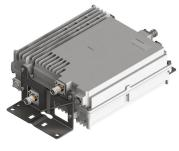
Tri Band Tower Mounted Amplifier, 1800/2100/2300 MHz, 12 dB, 2 BTS & 2 ANT ports, AISG with 1 RET connector (3 devices with 2 sub-units each), with 4.3-10 connectors
