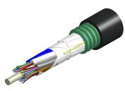
Fiber indoor/outdoor cable, LazrSPEED®, Single Jacket/Single Armor, 120 min Fire Survival, LSZH, 96 fiber, Gel-Filled, Stranded Loose Tube, Multimode OM4, Meters jacket marking, Black jacket color. Provides Rodent Resistance
