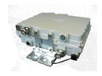
Dual Band Tower Mounted Amplifier, 1800//2600 MHz, 12 dB, 2 BTS & 4 ANT ports, AISG with 1 RET connector (2 device with 2 sub-units); with improved Out of Band Tx rejection
