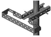
PIM-Guard® Antenna and RRU Cable Support Bracket with 23 ports for stackable hangers (up to 3 per port). Install with torque wrench set at 10 to 15 ft-lb to meet carrier PIM requirements. For patents, see www.cs-pat. com
