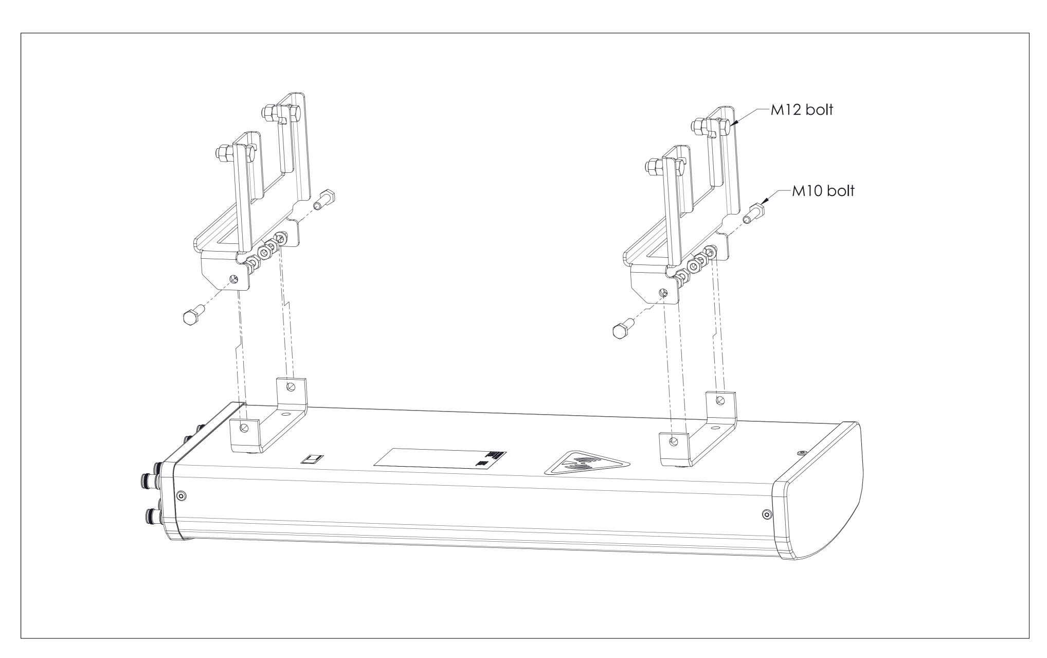
Assemble the antenna assembly by field installer
