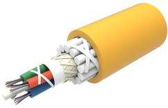
Fiber Indoor/Outdoor Cable, 24-fiber, Singlemode OS2, ULSZH, loose tube, gel-filled, Singlemode G.652.D and G.657.A1, Meters jacket marking, Yellow jacket color, Eca Flame rating
