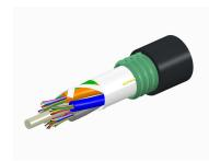
Fiber indoor/outdoor cable, TeraSPEED®, Single Jacket/Single Armor, Low Smoke Zero Halogen (LSZH), Singlemode G.652.D and G.657.A1, 12 fiber, Gel-Free, Stranded Loose Tube, Meters jacket marking, Black jacket color
