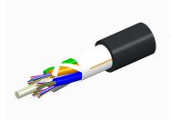
Fiber OSP cable, LightScope ZWP® Single Jacket All-Dielectric, 48 fiber, Gel-Free, Stranded Loose Tube, Singlemode G.652.D and G.657.A1, Meters jacket marking, Black jacket color
