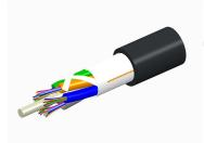
Fiber indoor/outdoor cable, TeraSPEED®, Single Jacket All-Dielectric (LSZH), 144 fiber, Singlemode G.652.D and G.657.A1Gel-Free, Stranded Loose Tube, Black jacket color, Meters cable marking, Eca flame rating
