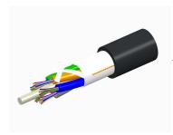
Fiber indoor/outdoor cable, LazrSPEED®, Single Jacket All-Dielectric, Low Smoke Zero Halogen (LSZH), Gel-Free, Stranded Loose Tube, 12 fiber, Multimode OM3, Black jacket color, Meters cable marking, Eca flame rating
