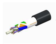
Fiber indoor/outdoor cable, LazrSPEED®, Single Jacket All-Dielectric, Low Smoke Zero Halogen (LSZH), Gel-Free, Stranded Loose Tube, 36 fiber, Multimode OM3, Black jacket color, Meters cable marking, Eca flame rating
