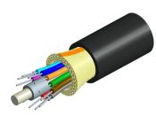
Fiber indoor/outdoor cable TeraSPEED® Indoor/Outdoor Plenum Distribution, 8 fiber single-unit, Singlemode G.652.D and G.657.A1, Gelfree, Feet jacket marking, black jacket color
