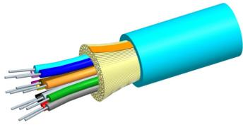
Fiber Indoor/Outdoor cable, Low Smoke Zero Halogen, Distribution, Gel-Free, 24 fiber single-unit, Multimode OM4, Meters jacket marking, Aqua jacket color
