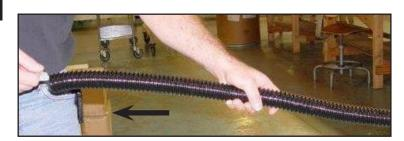
Remove electrical tape from the trunk cable and corrugated protection tube. While holding the protection tube straight pull the tube away from cable.
