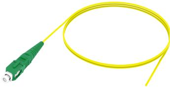
Fiber Optic Pigtail, Simplex, Singlemode, SC/APC to Stub, 0.9 mm diameter, 2 m
