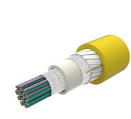
Fiber indoor cable, All-Dielectric, LSZH/Riser-Rated, Gel-Free, Central Tube 200µm Rollable Ribbon, 864 fiber, Singlemode G.657.A2/B2, Feet jacket marking, Yellow jacket color, Cca flame rating
