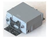
Dual Band Tower Mounted Amplifier, 700//850 MHz, 17 dB, 2 BTS & 2 ANT ports, AISG with 1 RET connector (1 devices with 4 sub-units), with 4.3-10 connectors
