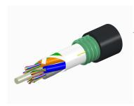
Fiber OSP cable, LightScope ZWP® Single Jacket/Single Armor, 288 fiber, Gel-Free, Stranded Loose Tube, Singlemode G.652.D and G.657.Al, Meters jacket marking, Black jacket color
