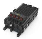
Mini-OTE 300-Series, Optical Terminal Enclosure, 4-port prodigy connector, with integrated 1x4 splitter, black, with grounding, external mounting. Splitter outputs connected to terminal housing ports, maximum 26 splices.
