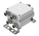
Twin Diplexer, 703-768 / 791-960 MHz, DC Bypass on low band port of Module 1 and high band port of Module 2, 7/16 DIN connectors
