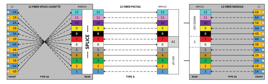
LC Method B Enhanced Polarity, Cassette to Cassette (2x12f splices)
