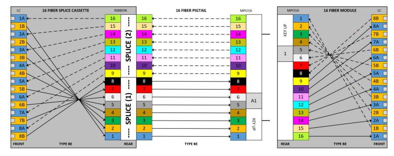
MPO Method B Enhanced Polarity, Cassette to Cassette (4x8f splices)
