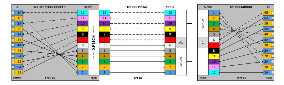
MPO Method B Enhanced Polarity, Cassette to Cassette (2x12f splices)
