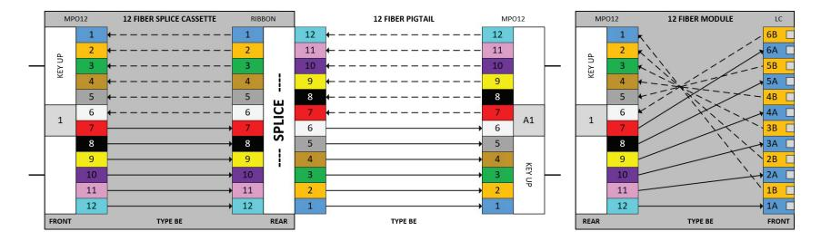
LC Method B Enhanced Polarity, Cassette to Cassette (4x8f splices)
