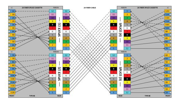
24f Cassettes LC Method B Enhanced Polarity, Cassette to two MPO12 Pigtail (2x12f splices)
