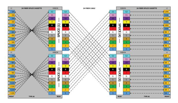
24f Cassettes LC Method A Polarity, Cassette to two MPO12 Pigtails (2x12f splices)
