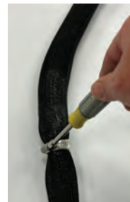
e) Remove tape covering cable clamp and remove clamp with socket tool.
