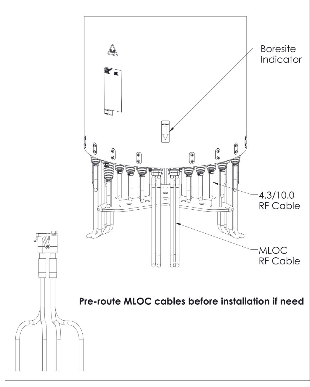
Figure 4. Routing Cables
