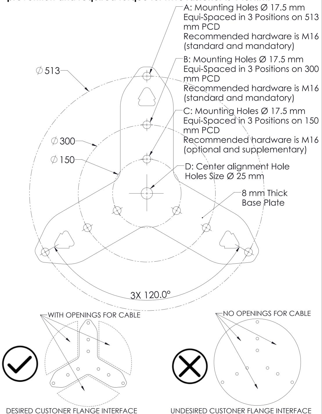
Figure 2. Mounting Interfaces on Base Plate Viewed From Bottom Side of Antenna
