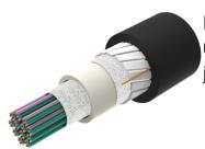
Fiber indoor/outdoor cable, All-Dielectric, LSZH, Riser-Rated, Gel-Free, Central Tube Rollable Ribbon, 864 fiber, Singlemode G.657.A2/B2, Feet jacket marking, Black jacket color, Cca flame rating
