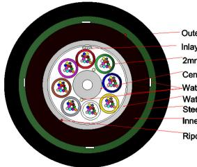
Outer Jacket PE /2mm Inlay Measuring Tape 2mm Stranded Gel Loose Tube / 12F Central Strength Member Water Blocking Tape/Yarns Water Blocking E-Glass Yarn Steel armoure Tape Inner PE Jacket / 1.7mm Ripcord
