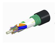
Fiber OSP cable, TeraSPEED® Single Jacket/Single Armor, Gel-Free, 6 fibers, Stranded Loose Tube, Singlemode G.652.D and G.657.A1, Feet jacket marking, Black jacket color
