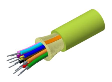
Distribution cables are color coded 900um tight buffered fibers for easy connectorization. Fiber counts above 24 are unitized for manageability. All fiber types are bend insensitive. Singlemode fiber is ITU-T G.657.A1 compliant as well as backwards compatible to G.652.D
